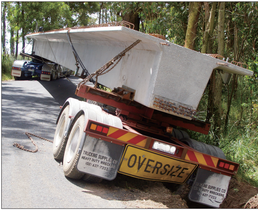
A prime mover and trailer literally sank into the road edge of Beards Trk on Wednesday afternoon. The trailer was loaded with a concrete bridge span about 25 metres long.
